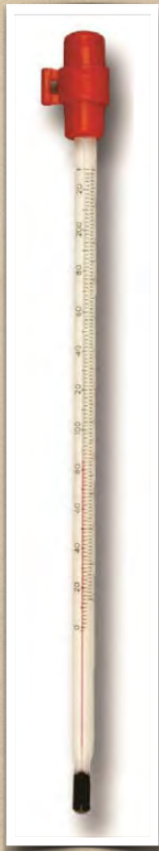
Mercury (silver) or alcohol (red) column thermometer
